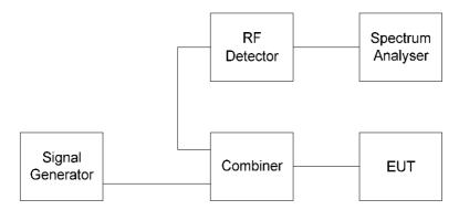
Figure 8: Measurement arrangement
