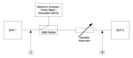
Figure 7: APC Measurement Setup
