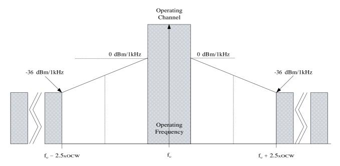
Figure 4: Out-of-Band Domain for Operating Channel
