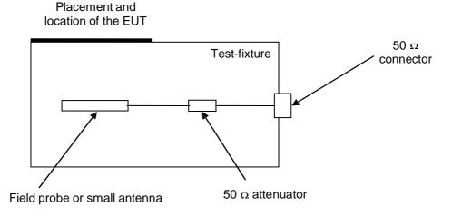
Figure C.1: Test fixture
