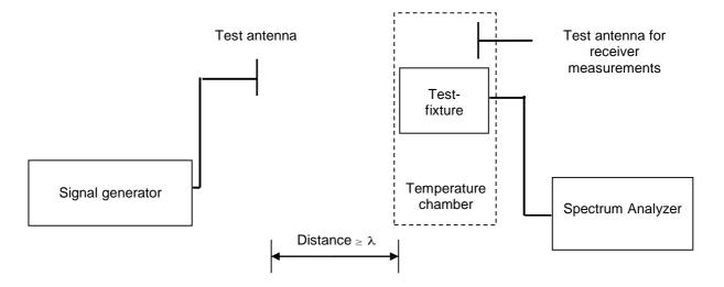
Figure C.2: Validation of test set-up without EUT
