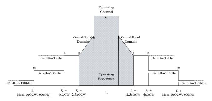
Figure 6: Spectrum Mask for Unwanted Emissions in the Spurious Domain
