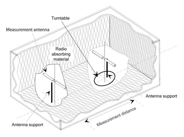
Figure B.3: A typical Fully Anechoic Room
