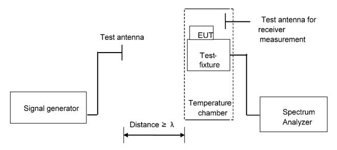
Figure C.3: Validation of test set-up with EUT in place
