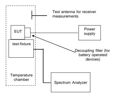
Figure C.4: Test of EUT
