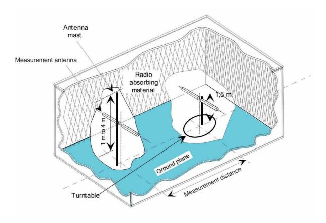
Figure B.2: A typical Semi Anechoic Room
