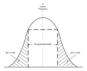
Figure 2: Signal Occupied Bandwidth
